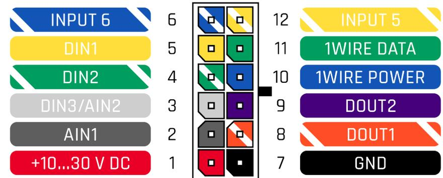
**Figure 2 FMB120 2x6 socket pinout**
