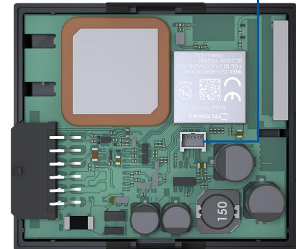
Figure 1 FMB120 device view
