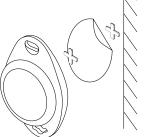
Using the adhesive sticker: Remove the release liner from one side of the adhesive sticker to stick it on the back of the device, then remove the release liner from the other side to stick it at the desired place on the wall
