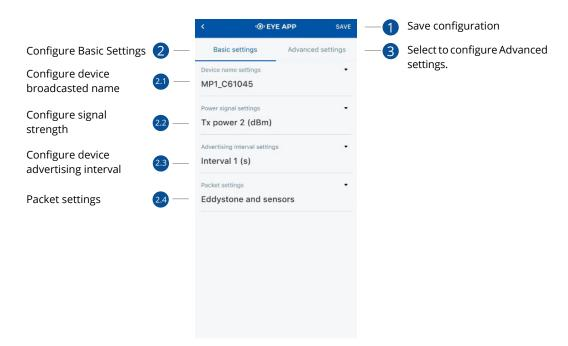
In this window you can check and change device configuration settings. In main tab Basic Settings (1) you can change main settings. Change Device name (2.1), Power signal strength (2.2), Advertising interval (2.3) and Packet (2.4) transmition type. For more settings go to Advanced settings (3) tab to enable various events.
