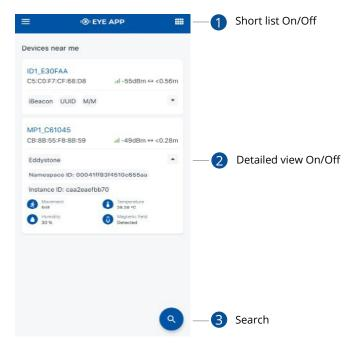
In this window you will see all visible devices. You have options to see devices in Short list (1) or in default list. When looking at devices in default list you will be able to open Detailed view (2) of devices and check transmitted data statuses. Additionally if you are looking for specific devices you will be able to use Search (3) function to filter search options. When in this window select a device of your choice to connect and after passing pin code you will go to device overview window.
