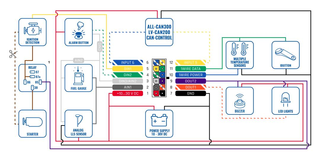
Figure 3 FMB120 Wiring scheme
