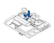
Figure 6 Battery connection
