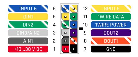
Figure 2 FMB120 2x6 socket pinout
