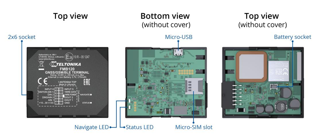
Figure 1 FMB120 device view
